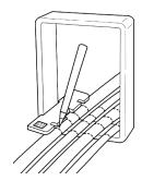
I. Pull the cables to final position. Put the EMC Marking Template in the frame with the yellow label facing you. Mark the cables.
