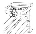
2. Attache the endpacking puller to the bolts with the nuts.
