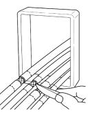
2. Remove the cable sheath between the two lines in the middle.
